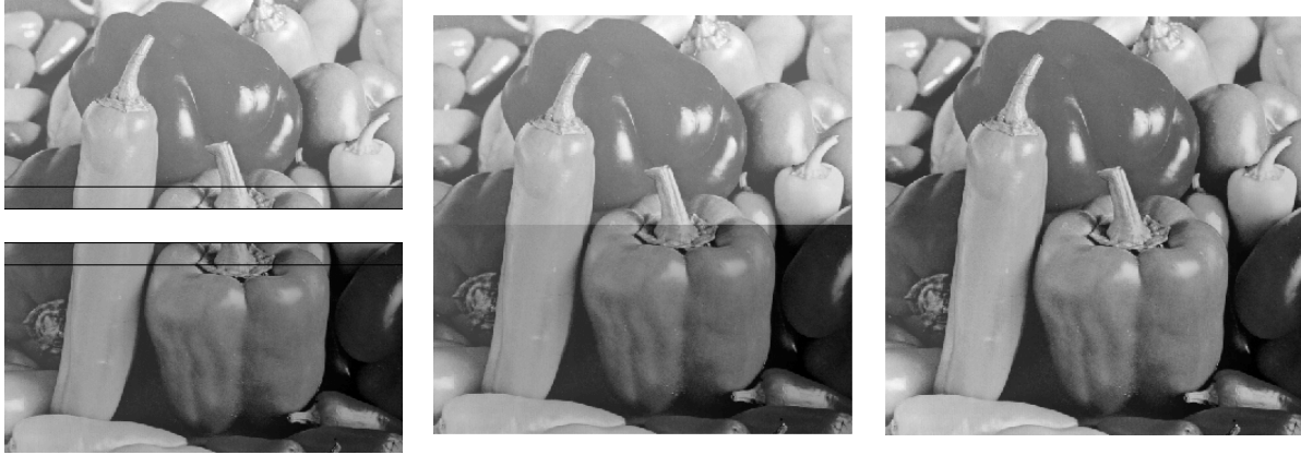
Fig. 2. Left to right: (a) Input images; (b) Direct pasting of intensities; (c) Result obtained using the proposed method. Mosaic image: 512 \times 512 pixels, overlap region: 30 pixels.
