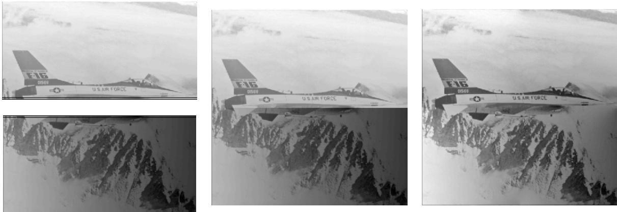
Fig. 5. From left to right: (a) Input images; (b) Direct pasting of intensities; (c) Result obtained using the proposed method. Mosaic image: 512 \times 512 pixels; overlap region height: 6 pixels.
